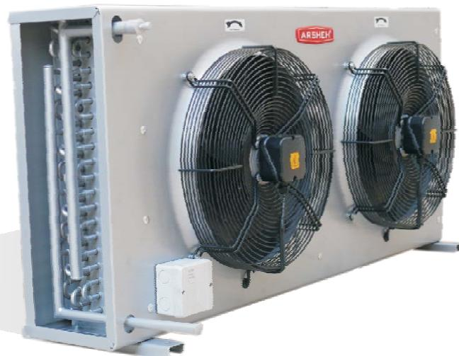
Our HCS -series condensers with **ARSHEHKAR** commercial brand are designed with 28 capacities ranging from 7.1 KW up to 172 KW. These condensers are utilized in ventilation and refrigerating systems. HCS -series condensers are compatible with R-22, R-134a, R-404A and R-407 C halocarbon refrigerants.
