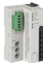
Remote I/O system
